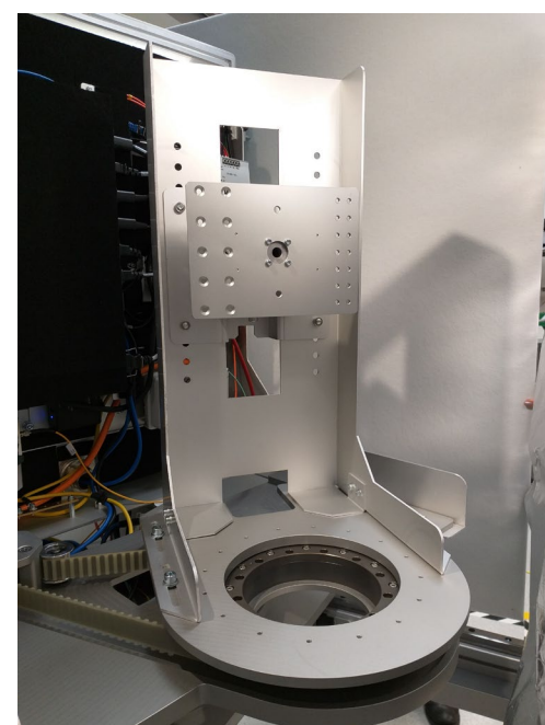
5G Antenna Positioning System
